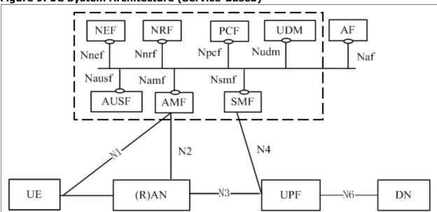
Figure 9: 5G System Architecture (Service-Based)
