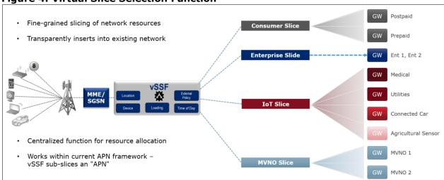
**Figure 4: Virtual Slice Selection Function**
