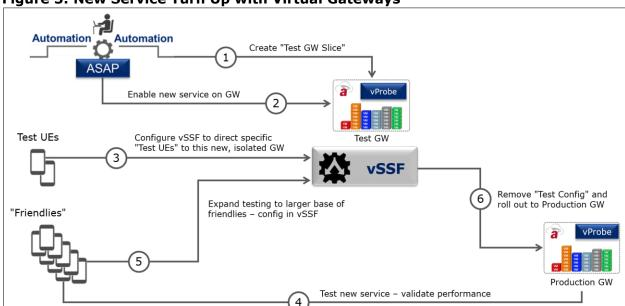
Figure 5: New Service Turn Up with Virtual Gateways
