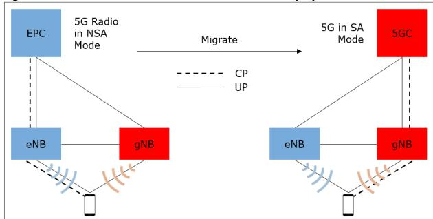
Figure 7: Non-Standalone & Standalone Modes for 5G Deployment
