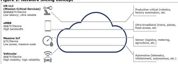
Figure 1: Network Slicing Concept
