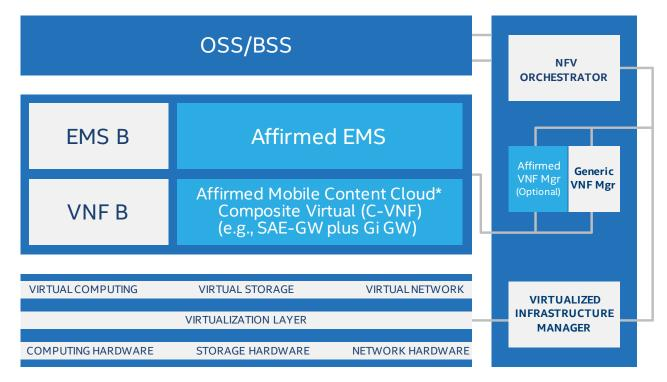
**Figure 2.** How Affirmed Networks\* Mobile Content Cloud\* fits into the framework. OSS/BSS: operations support system / business support system, EMS: element management system, VNF: virtualized network function.
