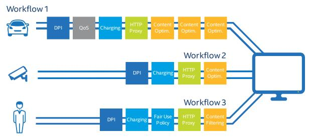
**Figure 4.** The Affirmed Services Workflow Orchestration framework enables fast and easy creation of services. QoS: quality of service, MVNO: mobile virtual network operator, Optim: optimization, Adapt: adaptation.
