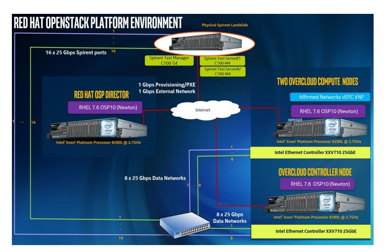
Figure 2. OpenStack Components
